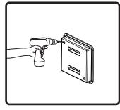
**7.** Insert speaker in hole. Tighten the two clamping screws. **DO NOT OVERTIGHTEN**.
